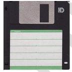
Floppy disks are small, removable, media storage devices. They record data onto a thin, circular magnetic film encased in a flat, square plastic jacket. Floppy disks are rarely used now, having been replaced by memory sticks and re-writable CD storage devices.
