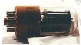
The first generation computers were huge, slow, expensive, and less reliable. Eckert and Mauchly built the ENIAC (Electronic Numerical Integrator and Calculator) computer which used vacuum tubes instead of the mechanical switches of the Mark I. The ENIAC used thousands of vacuum tubes, which took up a lot of space and gave off a great deal of heat just like electric
