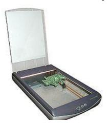
it to a digital image. Common examples found in offices are variations of the *desktop* (or flatbed) scanner where the document is placed on a glass window for scanning. Hand-held scanners, where the device is moved by hand, have evolved over time. Mechanically driven scanners that move the document are typically used for large-format documents, where a flatbed design would be impractical.
