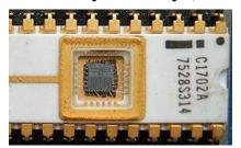
Read-only memory (ROM), also called Firmware are chips that store permanent instructions. Firmware boots up computerized or digital devices, as ROM chips are non-volatile, meaning they do not require a power source to hold their contents. This differentiates firmware from random access memory (RAM), which loses stored data at shutdown. Perhaps the most familiar firmware is the *basic*
